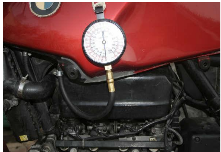
Testing the pump pressure
